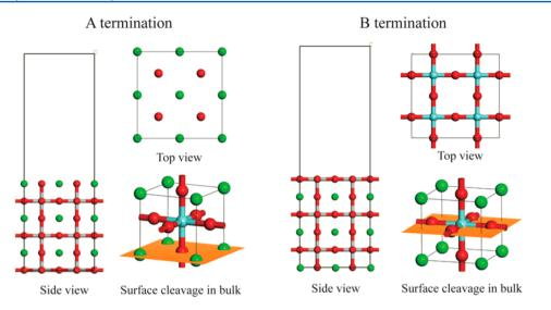
Figure 1. Atomistic models of the SrTiO<sub>3</sub>(100) surface of A termination and B termination. Color code: Sr, green; Ti, cyan; O, red.
