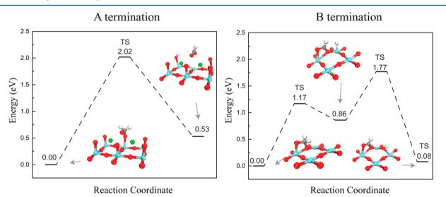
Figure 4. Second C–H bond activation of methoxy groups on  $SrTiO_3(100)$  of A termination and B termination. Color code: Sr, green; Ti, cyan; O, red; C, gray; H, white. Only the surface layer is shown.
