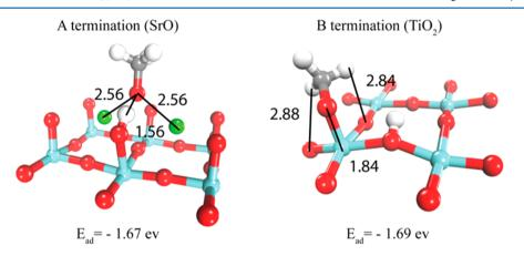
Figure 2. Dissociative methanol adsorption on the SrTiO<sub>3</sub>(100) surface's A termination and B termination. Key distances are given in Å. Color code: Sr, green; Ti, cyan; O, red; C, gray; H, white. Only the surface layer is shown.
