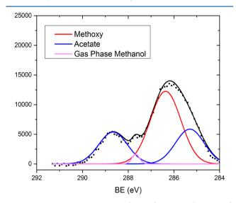
**Figure 8.** C 1s ambient-pressure XPS (APXPS) spectrum (dotted line) of a SrTiO<sub>3</sub>(100) surface at 250  $^{\circ}$ C after the addition of 0.1 Torr of methanol. The total fitted spectrum (black line) is from summing up the contributions from acetate (blue line), methoxy (red line), and gas-phase methanol (pink line).
