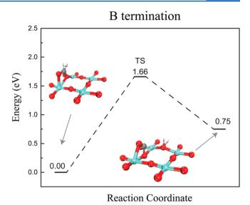
**Figure 5.** Third C–H bond activation of  $CH_3O$  on the  $SrTiO_3(100)$  B termination. Color code: Ti, cyan; O, red; C, gray; H, white. Only the surface layer is shown.
