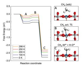
Fig. 5 Free energy profile of CH<sub>4</sub> activation on Pt<sub>1</sub>-rutile-TiO<sub>2</sub>(110) for a range of temperatures from 0 to 298 K. The structures for the initial state (A), transition state (B), and final state (C) are shown on the right. The free energies are obtained by including the zero point and vibrational contributions. The vibrational frequencies are obtained from the DFT calculations.
