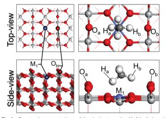
Fig. 1 Structural representations of the single-atom site,  $M_1$  (blue), doped on the rutile  ${\rm TiO_2(110)}$  surface (left) and  ${\rm CH_4}$  adsorption on the site (right). Ti, grey; O, red; C, dark grey; H, white.
