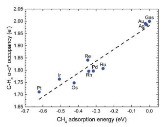
Fig. 4 Linear correlation between methane  $C-H_a \sigma - \sigma^*$  occupancy and adsorption energy on the M<sub>1</sub> (single-atom) site on rutile TiO<sub>2</sub>(110) with M being various transition metals.
