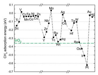
Fig. 2 Adsorption energies of methane on the  $\rm M_1$  (single-atom) site on rutile  $\rm TiO_2(110)$  with M being 3d, 4d, and 5d transition metals, in comparison with that on rutile  $\rm IrO_2(110)$  (green line). The Ti datum represents the undoped rutile  $\rm TiO_2(110)$ .
